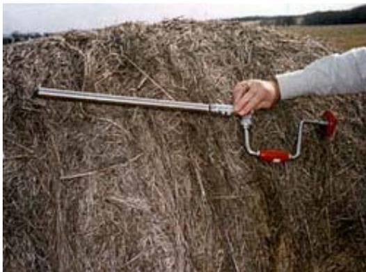
Figure 3 Hay corer attached to a manual hand drill (Photo: The Samuel Roberts Nobel Foundation)
